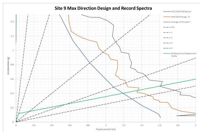
Figure 1: ADRS for Site 9 Building, showing the effect of scaling on building displacement
