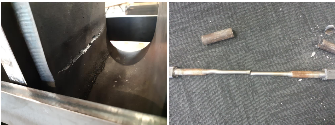
Figure 2: Additional effects found in energy-absorbing devices discovered in recent Dunning Thornton projects: Premature UFP failure from being cut across the steel sheet, early strain to failure of longer mini-BRB's.
