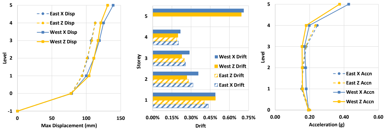
Figure 6. centre-of-mass average maximum response profiles (a) peak floor displacement (b) storey drift (c) peak floor acceleration
