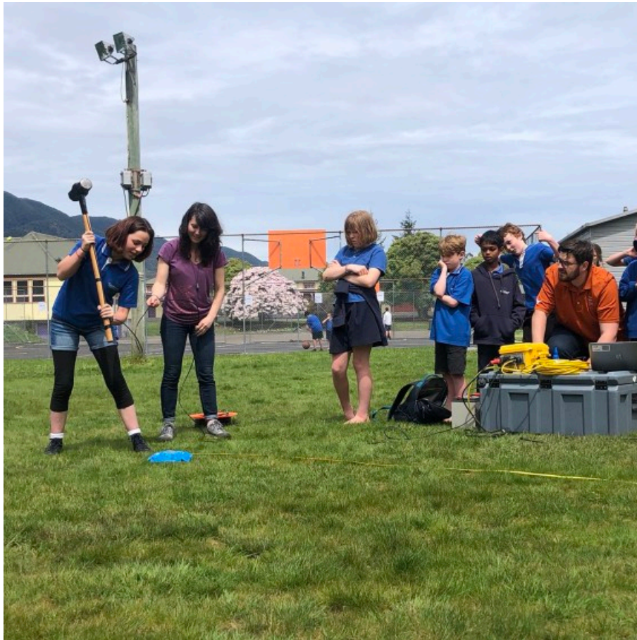
Figure 5: Dr Andrew Stolte demonstrates the MASW testing method to the students at Murchison Area School
