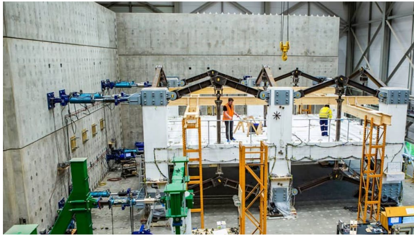
Figure 6: Global view of the building sub-assembly tested during the Recast floor project.
