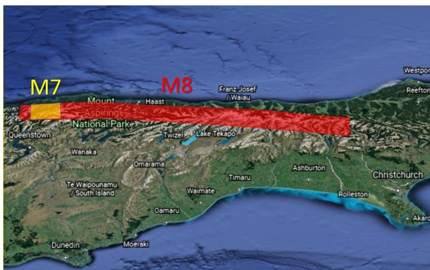
Figure 1: Comparison of hypothetical M7 and M8 earthquake rupture areas on the Alpine Fault.
