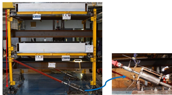
Figure 6: Constructed test building frame was retrofitted with two D3 viscous damper prototype as shown in the full-scale (left) and the D3 device up close (right).
