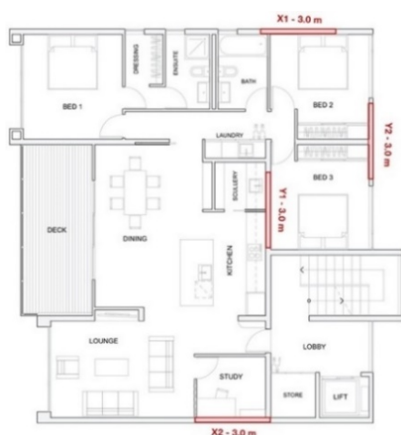
Figure 2: RC wall layout for Wellington case study building for code compliant design (Carradine, 2019).
