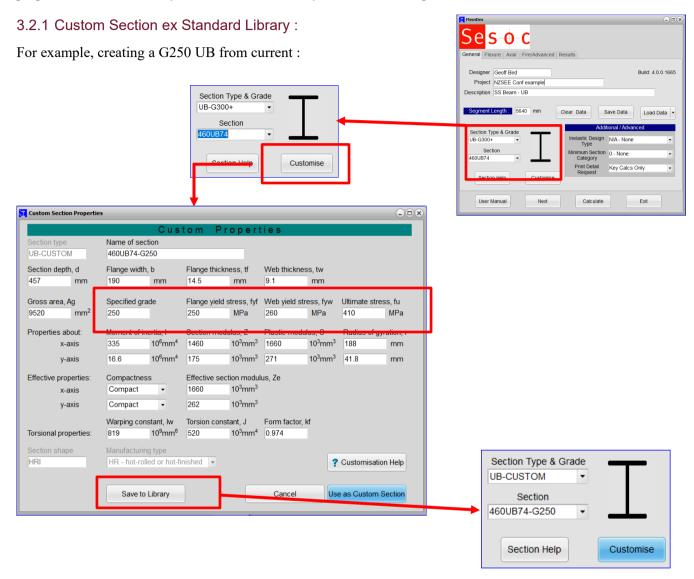
As the knowledgeable designer will be aware, some of the section design parameters are inter-related, e.g. steel grade & yield affects element slenderness ratios and potentially the effective section modulus, etc. It is thus incumbent on the designer, when using the CSLS capability, to ensure that all relevant provisions of NZS3404 are complied with.
