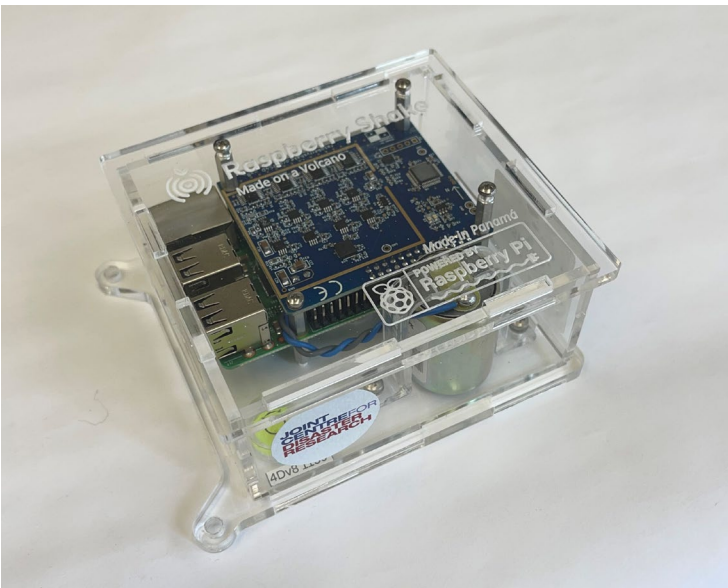
Figure 2: A Raspberry Shake seismograph in a standard clear acrylic case. The brass cylinder frame contains the geophone. The green board in the case is the Raspberry Pi computer, and the Raspberry Shake header board sits atop it. Credit: Lucy Kaiser
