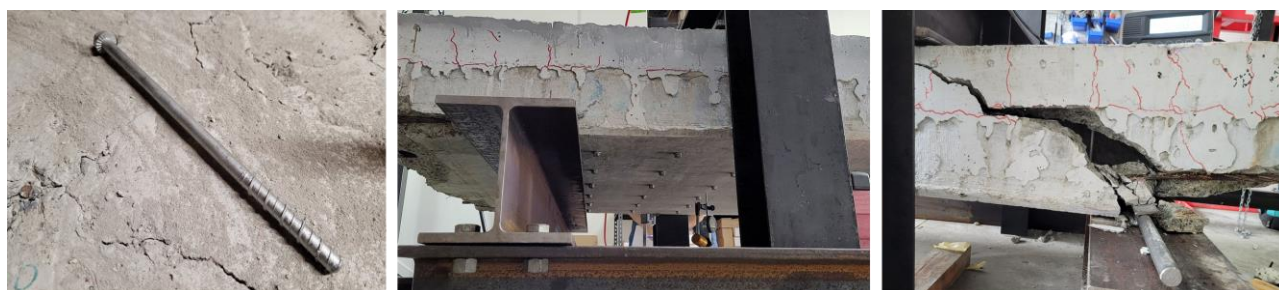
Figure 2: PYTHON HC fixing, strengthening configuration, and tested HC2 specimen
