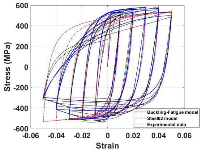
Figure 2. 6D-500E rebar stress-strain response
