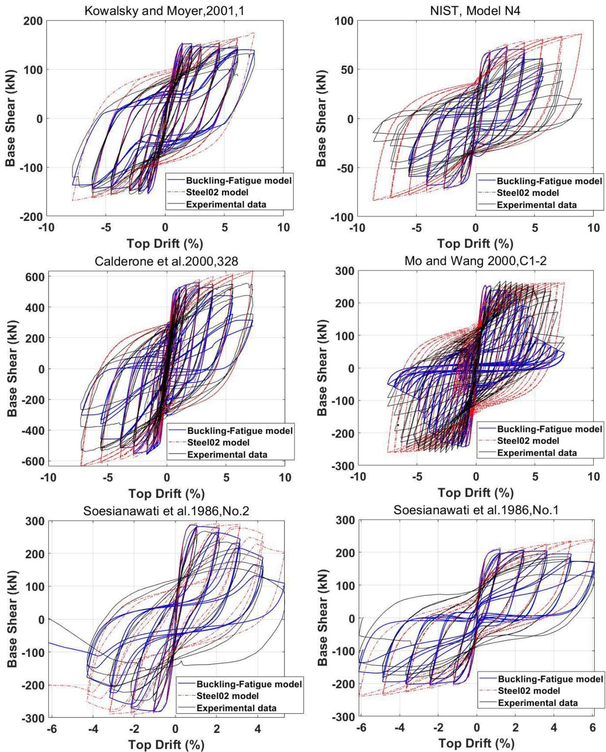
Figure 6: Force-displacement response of RC Columns
