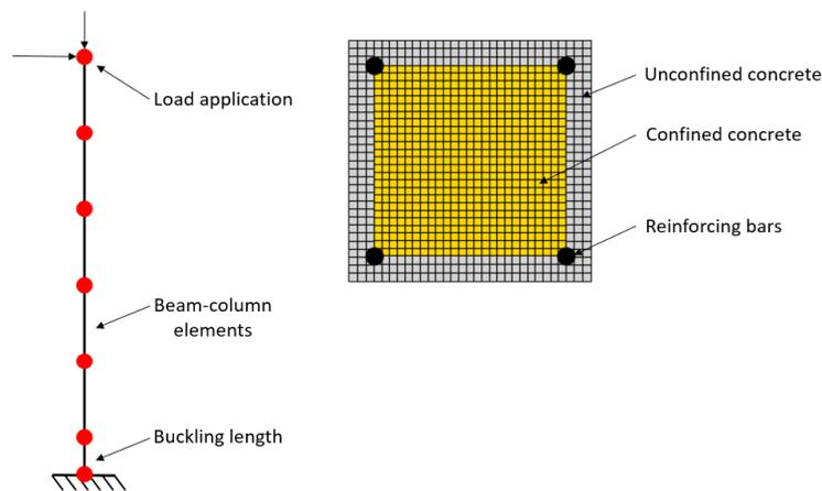
Saatcioglu and Razvi (1992). The cyclic behaviour of steel reinforcing bars is simulated by using the newly-implemented buckling-fatigue model or the pre-existing Steel02 material model.
