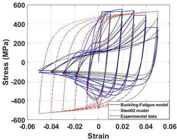
Figure 1. 15D-500E rebar stress-strain response
