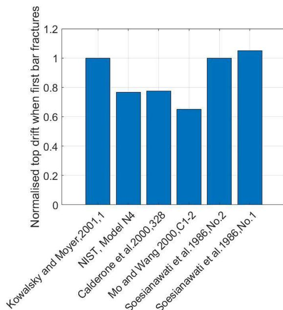
*Figure 7: Normalised top drift when first bar fractures*
