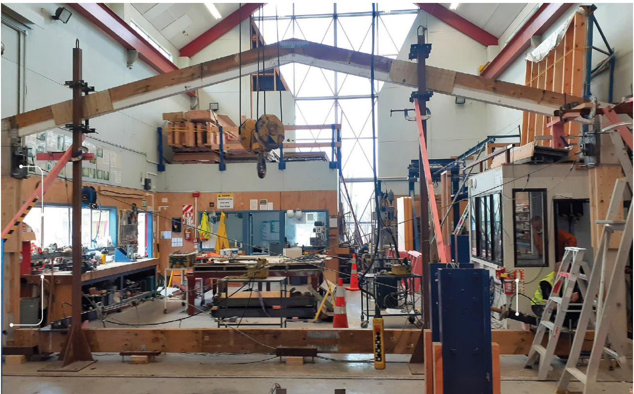
Figure 7 – BRANZ Structures Lab set up to test CEBUS portal frames
