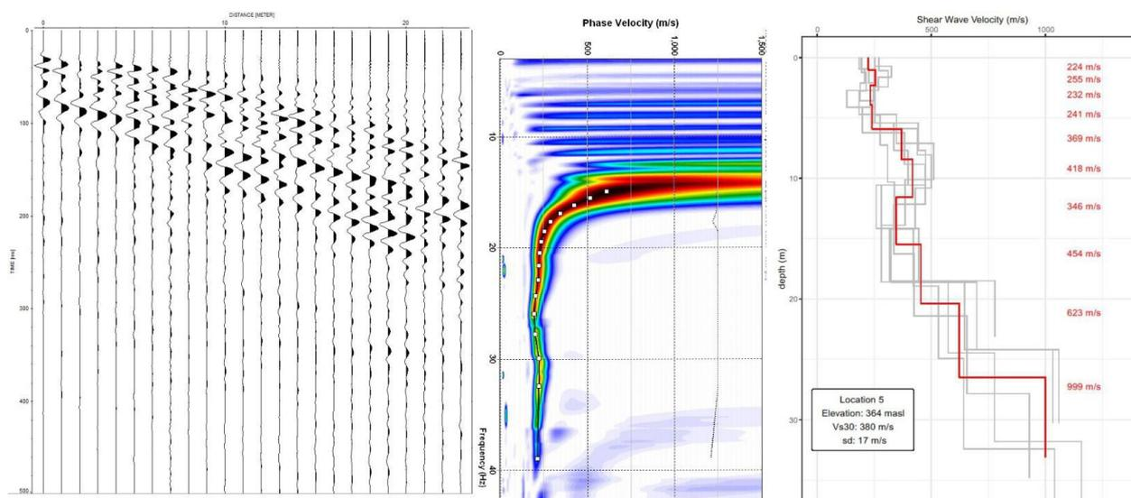
Figure 3: Example of MASW data. Left: seismic record as acquired in the field; Middle: dispersion spectrum with dispersion curve of fundamental mode picked; Right: A 10-layer Vs30 profile.
