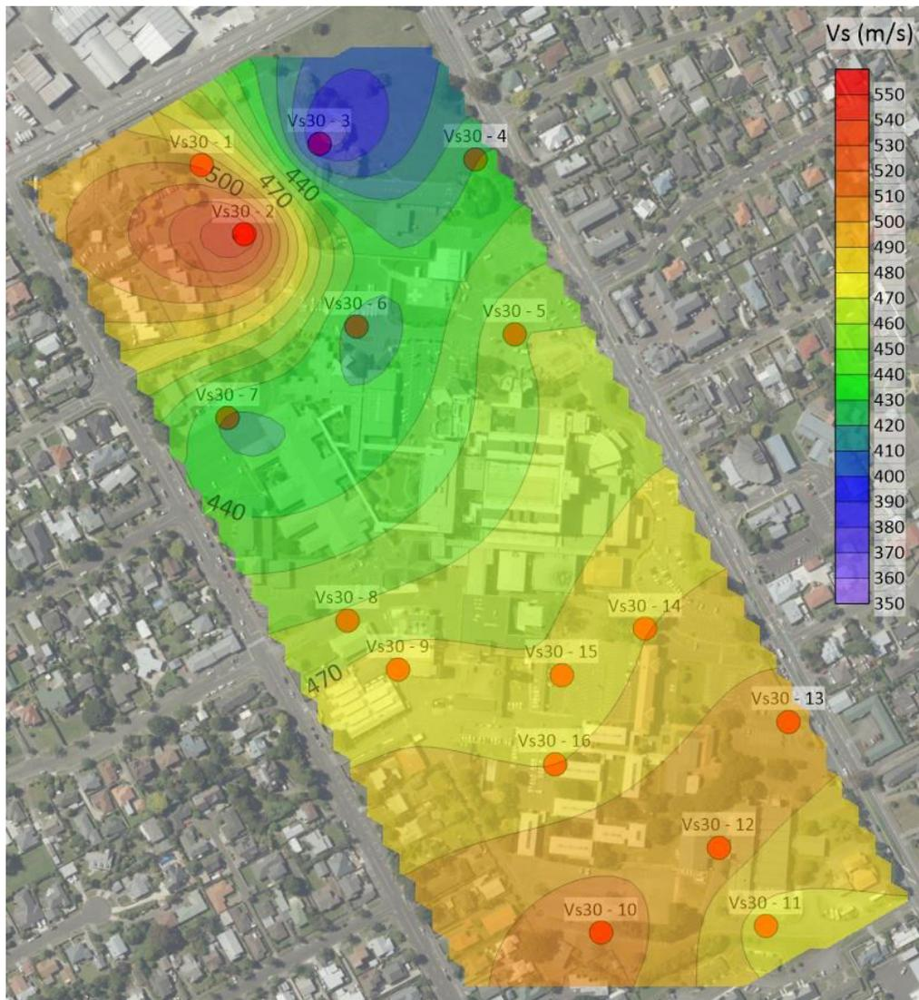
Figure 4: Example Vs30 contour map showing the variation in Vs30 values across a site.
