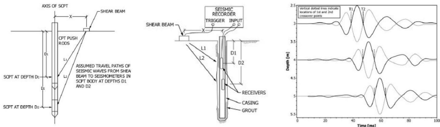
Figure 2: Diagram of SCPT data collection (left), diagram of DH Vs data collection (middle), and opposing polarity seismic waves at different depths (right) (modified from ASTM D7400 2017).
