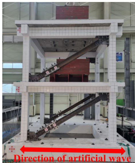
Figure 4: The RC frame with friction-damped diagonal brace. (RF)
