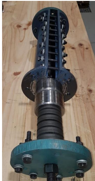
Figure 2. Self-centring Structural Connector (SSC).
