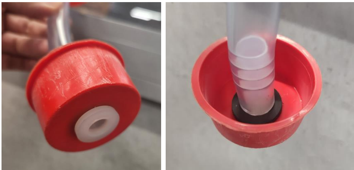
Figure 5: Underside of top-exit grout tube (left), top side of top-exit grout tube (right)
