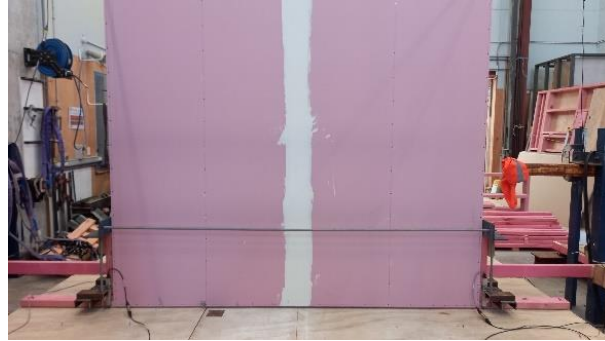
(c) Final appearance of the 2.4 m wall on suspended timber floor (perpendicular to joist orientation)
