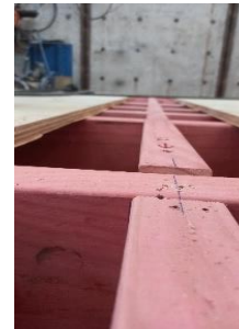
(b) Out-of-plane movement of the floor timber
