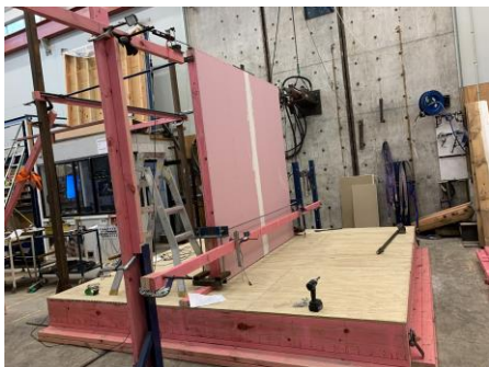
Figure 5. Test setup of LTF walls on suspended timber floors
