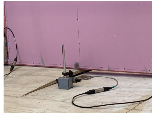
(b) Flooring lift up along the flooring joint
