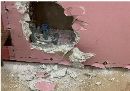
(c) Exposed view of Handibrac screw pulled out
